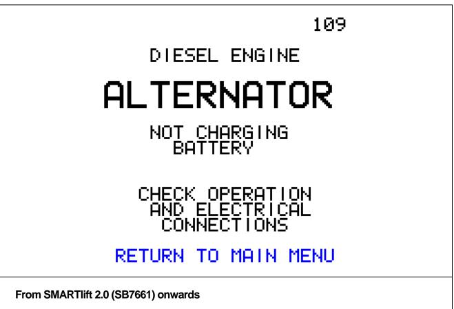
The Alternator on the Kubota Diesel Engine is not charging the battery.
