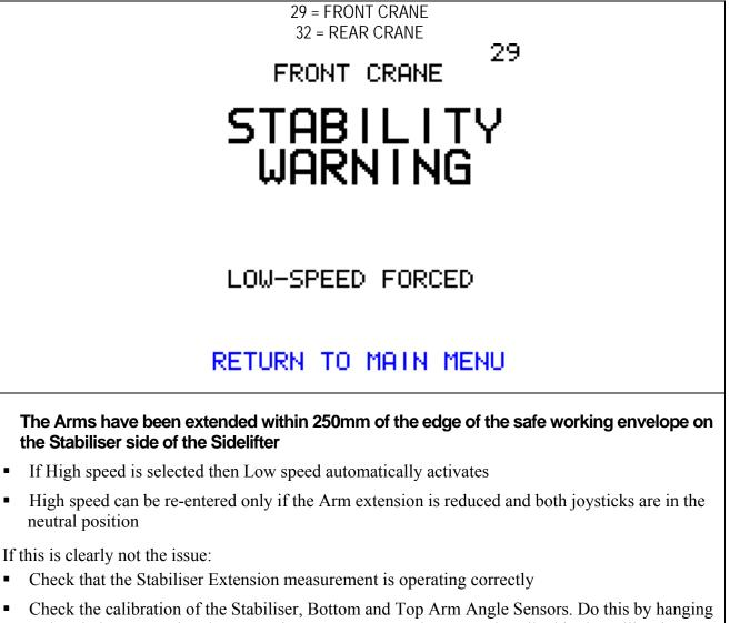
. a plum bob one at a time between pins A&D, D&G and H&L as described in the calibration procedure SL0005 2GB and then go to the MANUFACTURERS AREA then VIEW PIN **DISTANCES** and check that the HORIZONTAL DISTANCES, AD, DG and HL are zero mm  $(\pm 10 \text{mm})$  when the plumb bob is lined up
