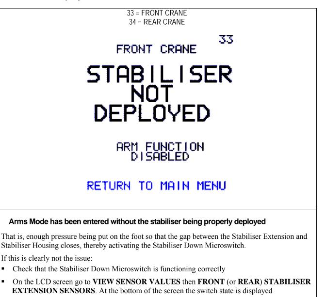
• With the Stabiliser on the ground NO = 1 and NC = 0, with the stabiliser foot not in contact with the ground NO = 0 and NC = 1
